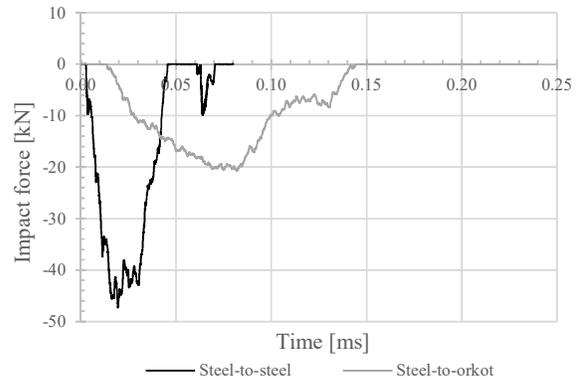
Figure 6: Impact force as a function of time (both at Model scale) for a conventional (steel-to-steel) and PULSE (steel-to-orkot) blow.
