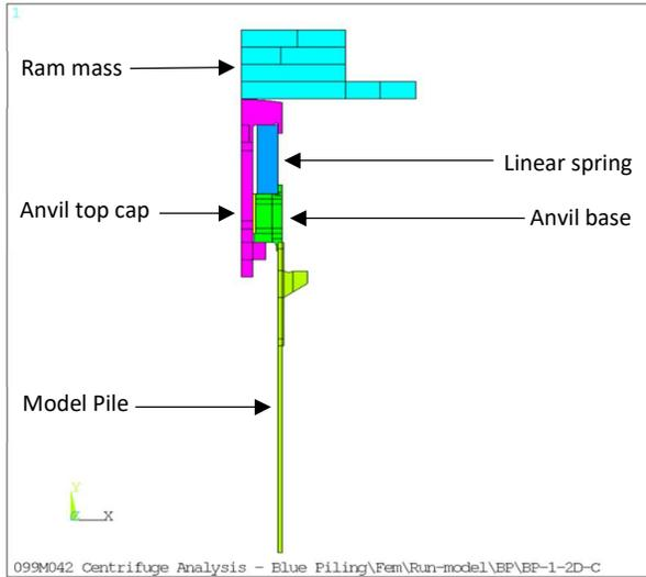
Figure 7: (Axisymmetric) model geometry of the numerical model used to simulate a BLUE Piling blow.
