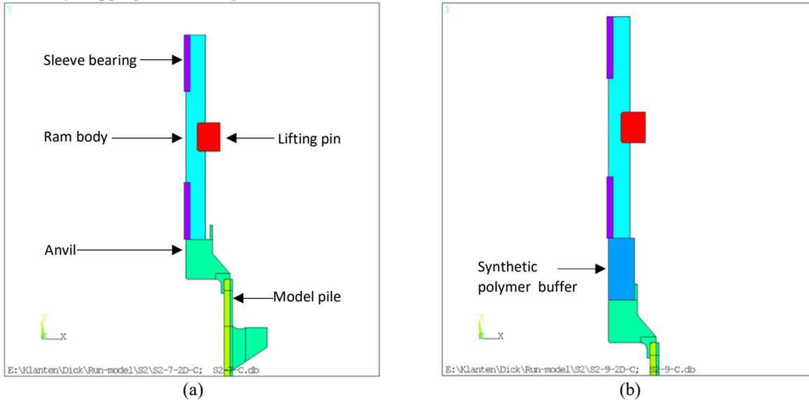
Figure 5: (Axisymmetric) model geometry of the numerical model used to simulate a conventional (a) and PULSE (b) blow in the centrifuge.
