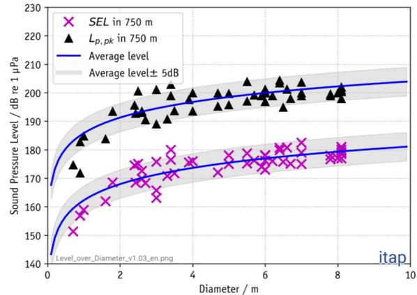
Figure 2: Recorded SPL as a function of pile diameter, at a distance of 750 m from the source. All piles were installed dynamically, without the application of technical noise abatement systems (Bellmann et al., 2020)
