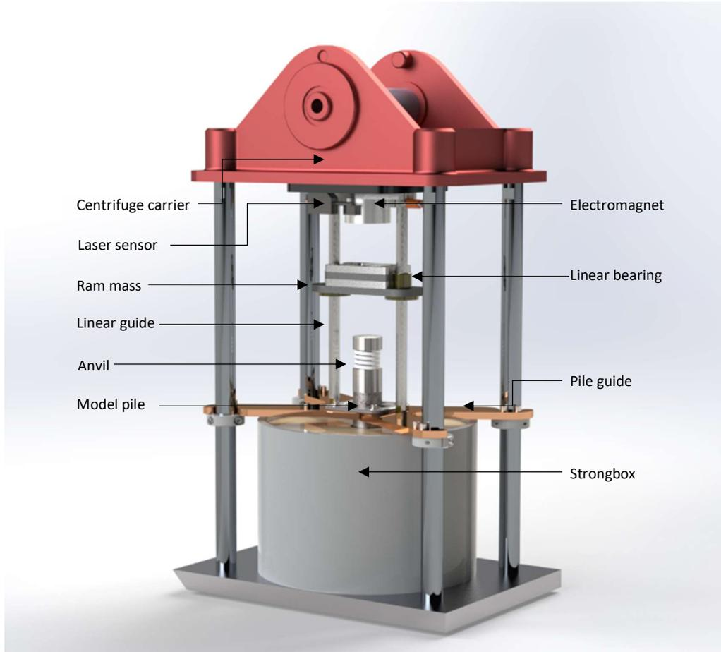
Figure 9: BLUE piling actuator for the centrifuge facility of DUT.
