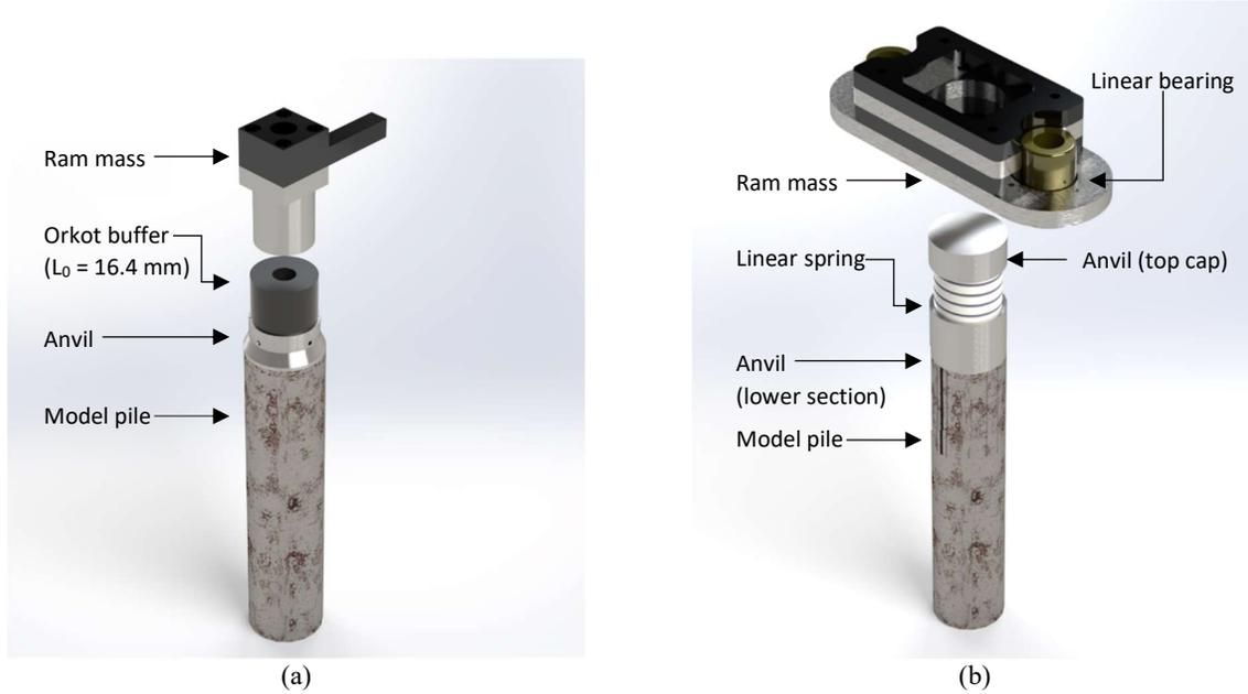
Figure 4: Pile assemblies for the replication of PULSE- (a) and BLUE-blow (b) characteristics in DUT's centrifuge facility.
