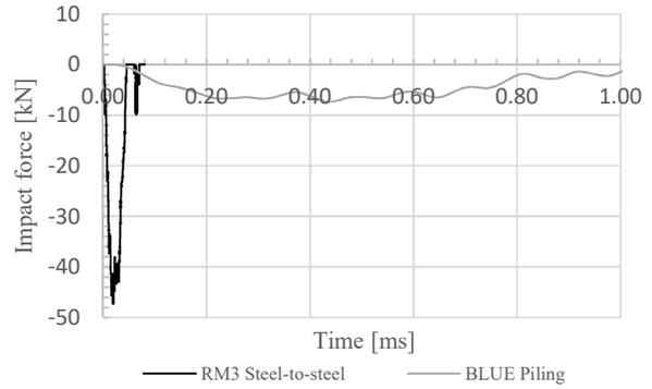
Figure 8: Impact force as a function of time (both at Model scale) for a conventional (steel-to-steel) and BLUE Piling blow.
