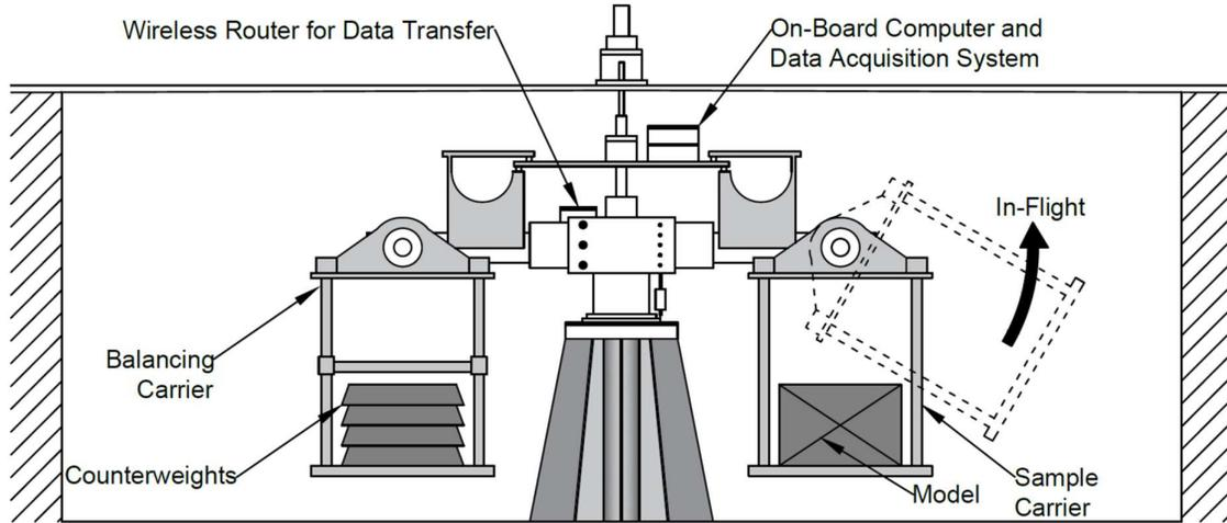
Figure 3: Schematic illustration of DUT beam centrifuge, adapted from Q. Li (2020).
