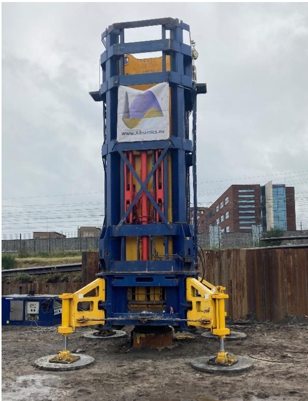
Fig. 7. Rapid Load Testing system StatRapid.
