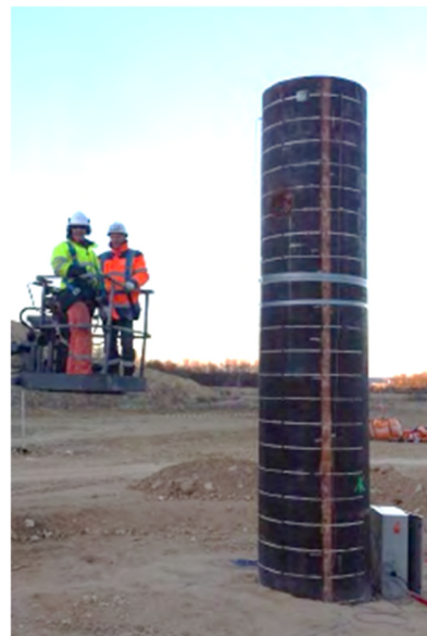
Fig. 1. Test setup with accelerometers and manually applied hammer stroke from a cherry picker
