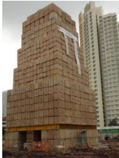
Figure 1. Massive Kentledge Test by Stacking Concrete Blocks
