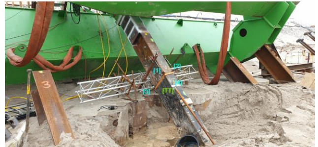
Fig. 7: Reaction frame, test pile in the centre, left reaction pile not visible, right reaction pile on the right in the picture.
